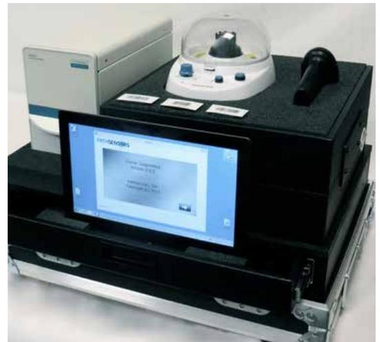
*PathSensors’ Zephyr pathogen identifier incorporates CANARY technology and provides rapid, sensitive and specific identification of biological threat agents (bacteria, viruses and toxins) from surface samples. Source: PathSensors.*
